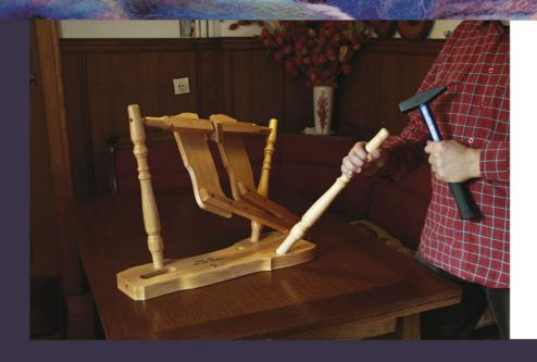
The first step is to attach the rear leg (the front legs and treadle assembly are already in place).
