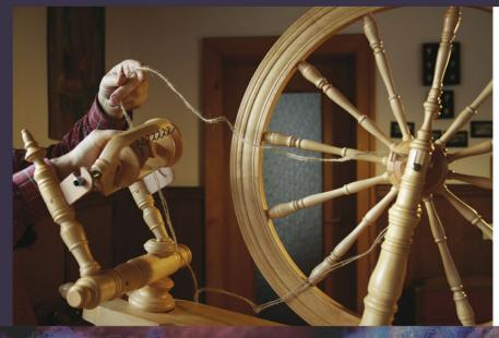
Place the drive band (two loops) around the wheel. To get the band in position it may be necessary to tighten or loosen the tension on the band by turning the tension adjusting knob at the end of the bench.
