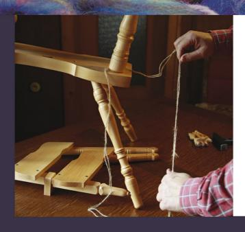
Prepare the drive band, by doubling, so that there are 2 loops, and drop it over the front wheel post.
