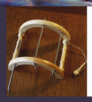
Your bobbins go on the metal rods with the brake band going over the pulleys that are at the end of each bobbin. Tighten the thumb screw as needed to create drag on the bobbins as you ply.
