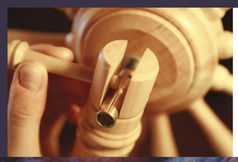
Secure the wheel axles with two wooden pegs, being sure to orient the small groove on the outside surface of the bearing on top. The wooden peg will slip along this groove as you push it in. Put the small hole (for oil) closest to the wheel hub.
