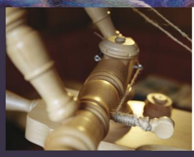
Attach the brake spring to the outside eye screw.
