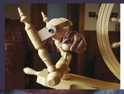
Place the Mother-of-All base over the threads on the wooden bolt. Attach the Mother-of-All nut. Do not tighten completely.
