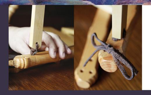
Thread both ends down through the larger hole on the treadle. Remove any slack. Pull the two ends up through the two remaining holes in the treadle, pull tightly again, then tie.
