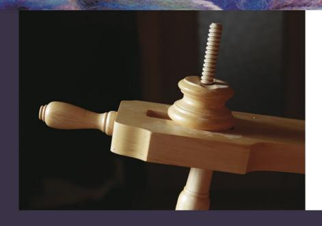
Place mother-of-all support into the wooden bolt. (This is the larger of the 2 wooden nuts.)
