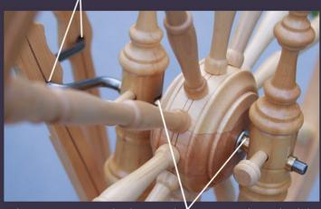
The two metal sleeve bearings that hold the axle; a small oil hole is on each for adding lubricant.
