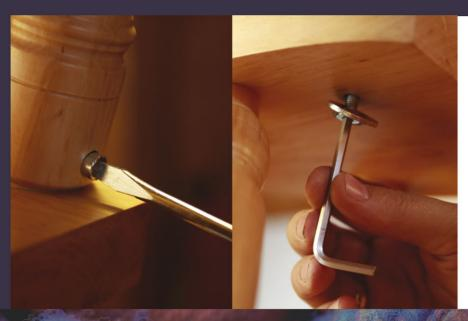
Take a barrel nut, bolt, a center ring and a washer. Use a screwdriver on nut to help line up hole. Snug, but do not completely tighten the bolt.
