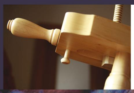
Insert the locking peg into the hole on the bottom of the bench so that it secures the tension screw.
