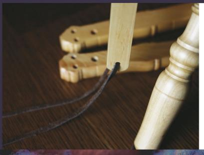
Loop a length of leather through the hole at the end of each footman and tie a firm square knot against the bottom of the footman.
