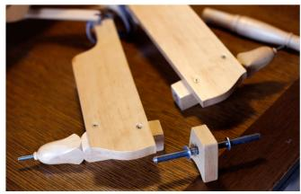
As it is shown in the picture, embrocate 1 - 2 minutes the thick bar connecting the treadles. It should be done carefully, to obtain thick layer of paraffin on the bar.
