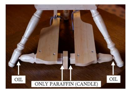
In all grease places of the Minstrel you should dose the oil added to the Minstrel. Apart from the metal connection of the traedles - YOU MUST NOT USE THE OIL. Otherwise, the spinning wheel will scrunch. Once for a couple months you have to wax by paraffin (candle) the bar.
