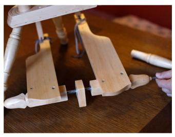
Then, pull out both treadles from spinning wheel's legs.
