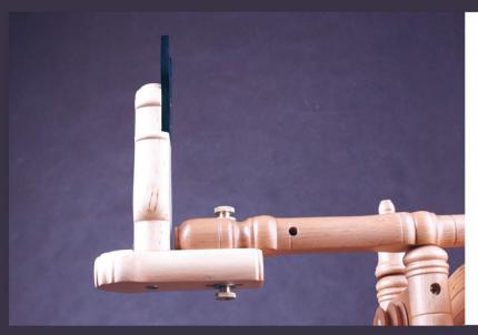
Install the Front Maiden Post with Base by placing the base on the underside of the Mother-of-All and screwing in the top and bottom brass knobs at the same time, as pictured below. Do NOT fully tighten at this point.
