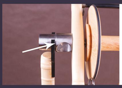
The last thing to check before tightening the brass knobs, is that the Flyer spins freely and smoothly when turned by hand. If there is any resistance or tightness felt when attempting to spin the Flyer by hand, adjust the slide slot on the Front Maiden base away from the drive wheel just a fraction to create a small gap between the graduated lip on the orifice and the Front Maiden bearing.
