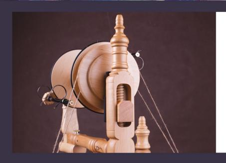
A correctly installed, best fitting drive band will look like this from the backside of the wheel. The tension on the drive band will be taut but not overly tightened. To adjust tension of your drive band turn the Tension Screw to move the Adjusting Block up and down until proper tension is achieved.
