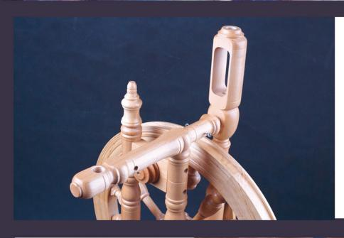
Once the components have been removed, the Mother-of-All unit will look like the wheel pictured left. Bring the drive band to the front of the wheel, over the Mother-of-All and store it away by wrapping around the bottom of the support posts and tying off, as pictured below.
