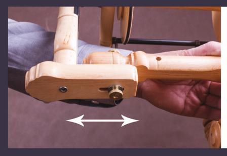
Once proper alignment is achieved, determine if you need to reduce the spacial play that may be between the Front Maiden bearing and the Adjusting Block bearing.
