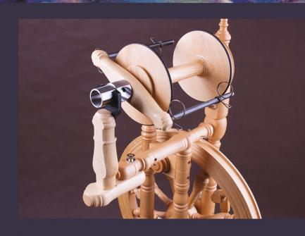
While twisting the Front Maiden with Base into a more perfect alignment with the Mother-of-All, insert the tip of the Flyer spindle into the groove of the Adjusting Block bearing.
