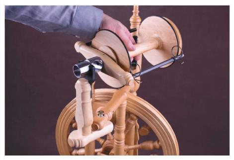
With the brass knobs still loose, angle the Front Maiden to one side and place the Flyer orifice into the Maiden bearing, ensuring that the graduated lip of the orifice is flush with the bearing.
