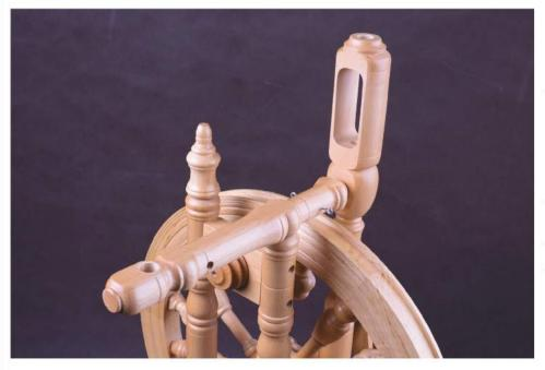
Once the components have been removed, the Mother-of-All unit will look like the wheel pictured left. Bring the drive band to the front of the wheel, over the Mother-of-All and store it away by wrapping around the bottom of the support posts and tying off, as pictured below.
