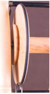
The last thing to check before tightening the brass knobs, is that the Flyer spins freely and smoothly when turned by hand. If there is any resistance or tightness felt when attempting to spin the Flyer by hand, adjust the slide slot on the Front Maiden base away from the drive wheel just a fraction to create a small gap between the graduated lip on the orifice and the Front Maiden bearing.
