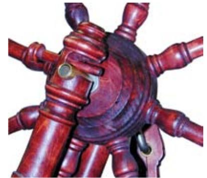
A small eye bolt should be installed in a pre-drilled hole at the front left of the mother-of-all; this is used to hang your threading hook. If you prefer a different location for this eye bolt, just move it. You can use the large hole in the bench to store your hook when not spinning.
