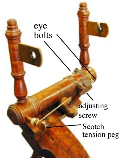
The Scotch tension is assembled in this manner: two eye hooks are placed on each side of the mother-of-all base in pre-drilled holes. The spring is attached to the far outside hook; the brake band is tied to the spring and will go up and over the bobbin pulley, down to the next hook, and then forward to the tension peg.
