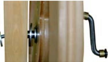
At the rear of the wheel you will see a metal shaft. On to this shaft slip on a smaller washer and then the larger washer. Fit the shaft through the hole in the wheel post and then secure with the 3 parts shown in picture below. Again, make this connection very snug. Rotate the wheel and note the ease of the spin.
