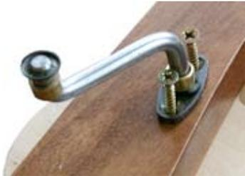
The front eye screw (on left side of tension arm) can be used to hang your threading hook.
