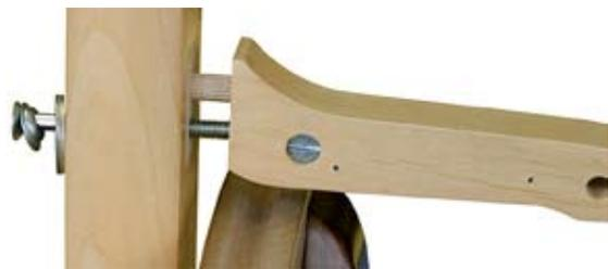
The metal handle uses 2 Phillips head bolts; tighten to pull the handle in snug to the post.
