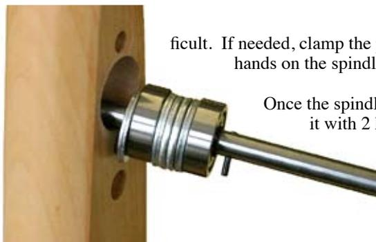
Once the spindle is seated in the hole you will secure it with 2 hex bolt units. Both ends have a hex head; the threaded bolt piece goes into the post from the front and the female piece is inserted from the rear. Using your hex wrench, pull the 2 parts to the post and make a snug fit. This
