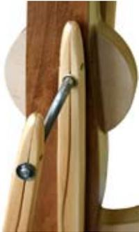
Place your elastic drive band over the wheel and post and allow to drape at the floor to the rear of the treadles. The drive band must be in position before you begin the next step.
