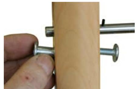
connection should never be loose but do not over tighten.
