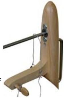
The Scotch tension brake band is adjusted with a small thumb peg. This peg can be positioned on either side of the tension arm. Tie the brake band to the thumb peg.
