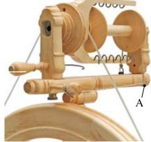
• mount the mother-of-all on top of the wheel post and secure with knob 2 at an angle that is perpendicular to the front face of the wheel. Never over tighten this connection as it may cause damage. Just tight enough to hold the part.
