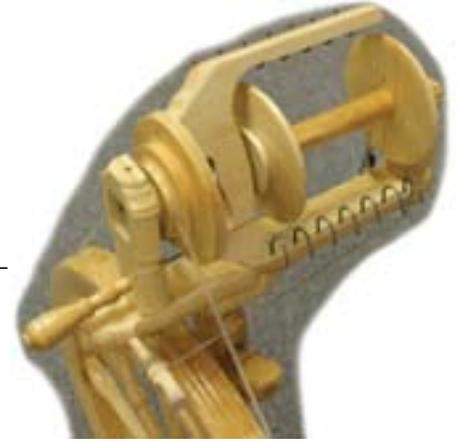
3. Mount the flyer on the 2 maiden posts in the normal fashion, being sure to snap the metal spindle into position on the rear maiden. There is a thin leather “thrust bearing” on the orifice; keep this in place when you mount the flyer. The mother-of-all should be at a perpendicular angle to the wheel; not twisted.
